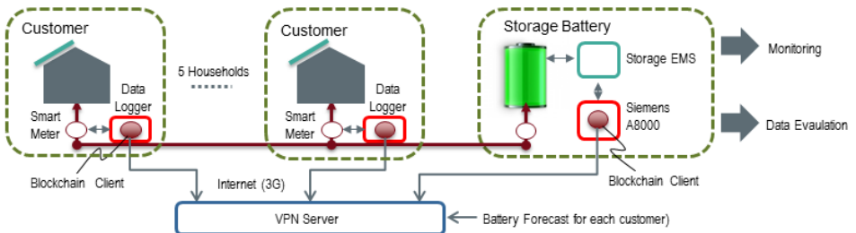
Figure 1. Battery Management Use Case Proof-of-Concept Architecture
