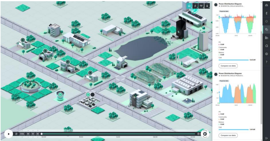
Figure 1: BIFROST UI: You can see an energy community scenario consisting of multiple different stakeholders (residential buildings, commercial buildings, battery storage), the simulation timeline at the bottom, and some simulation results on the right side.
